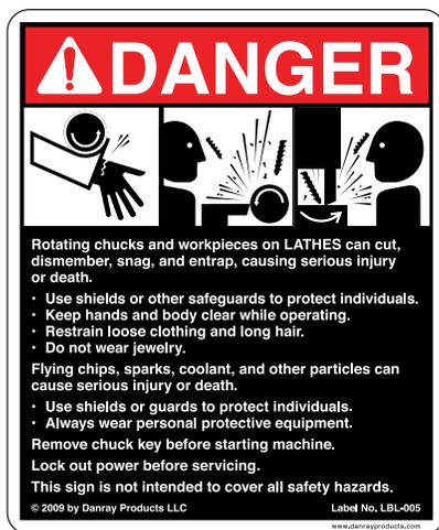
One LBL-005 sign is included with every shield assembly. Affix this sign to a prominent location on the machine so that it is easily seen and understood by individuals in the hazard area. Additional signs for other machinery and equipment are available as well as polycarbonate sign backings; contact us by phone, fax, e-mail, or online.
