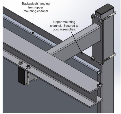
4. Backsplash panels may be removed as needed for machine setup or maintenance.
