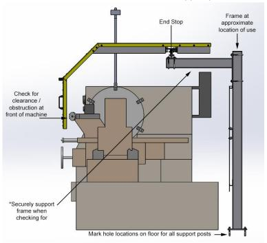
7) Secure support posts to floor using the ½"-13 x 3-3/4" Concrete Stud Anchors provided. Due to irregularities in floor, it is highly recommended to properly shim posts (shims not included) if required to insure secure and level anchoring to floor.
